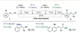
Fig. 2 Dual functionalization of aryl benzyl ethers in a one-flow microreactor via controlled sequential isomerization reactions.
