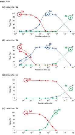
Fig. 1 Tandem isomerizations of various aryl benzyl ethers by changing the residence time in R1 in a flow microreactor system for products 2, 3 and 4d, followed by further stirring in a flask at 50 °C for 1 h to obtain products 4a-c (#). Methyl triflate was used as an electrophile (symbol ▲ with a dashed line), instead of methyl iodide (symbol • with a solid line).
