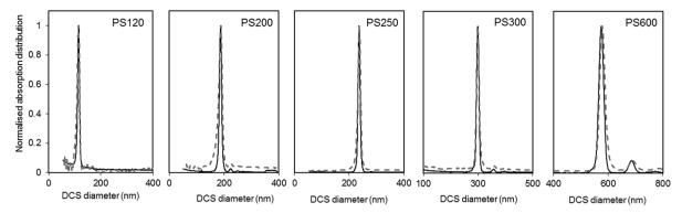
Fig. 3 Normalised light extinction weighted size distributions of the PS NPs as measured by DCS in sedimentation (continuous black line) and flotation (dash grey line) modes. The NPs are assumed perfect spheres of density as in Table 1.
