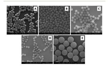
Fig. 2 Representative SEM images of PS NPs of samples (A) PS120, (B) PS200, (C) PS250, (D) PS300 and (E) PS600.
