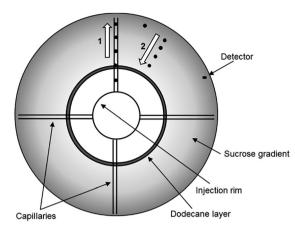
Fig. 1 Schematic representation of the principles of the functioning of the DCS disc for low density particles. The particles are injected in a rim and travel to the edge of the disc through four capillaries (1). From the edge, the particles float towards the centre of the disc through a sucrose gradient of higher density (2). The particles are detected when travelling in front of the detector.
