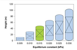
Fig. 2 Height of the absorber as a function of the chemical equilibrium constant of the solvent at 303 K. Green figure corresponds to the height of an absorber using 30 wt% MEA.
