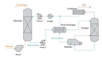
Fig. 1 Process flow diagram of the  ${\rm CO_2}$  absorption capture plant modelled in this work.
