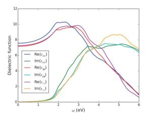
Fig. 13 Three components of the calculated dielectric function,  $\varepsilon(\omega)$ , as a function of incident photon energy,  $\omega$ , for bournonite (CuPbSbS<sub>3</sub>).
