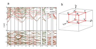
Fig. 11 Calculated band structure of bournonite (CuPbSbS<sub>3</sub>) showing the result without the inclusion of spin-orbit coupling (SOC) in green and the calculation including SOC in red (a) and the reciprocal space k-path for the structure determined by the Aflow-online utility<sup>74</sup> (b).
