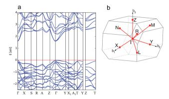
Fig. 8 Calculated electronic band structure of stephanite ( $Ag_SSbS_4$ ) (a) and the reciprocal space k-path for the structure determined by the Aflow-online utility<sup>74</sup> (b).
