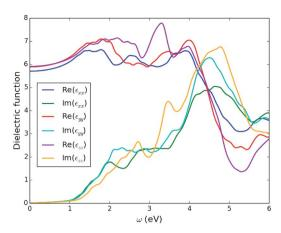
Fig. 6 Three independent components of the calculated optical dielectric tensor,  $\varepsilon(\omega)$ , as a function of incident photon energy,  $\omega$ , for enargite (Cu<sub>3</sub>AsS<sub>4</sub>).
