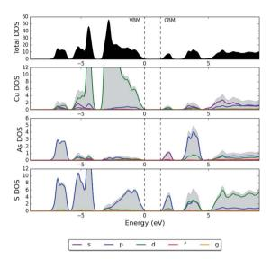
Fig. 4 HSE06 + SOC partial electronic density of states (pDOS) of enargite ( $Cu_3AsS_4$ ), where the top of the valence band has been set to 0 eV.
