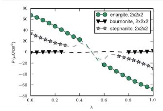
Fig. 14 Spontaneous polarisation along a path connecting the structures with  $+P_s$  and  $-P_s$  for enargite (Cu<sub>3</sub>AsS<sub>4</sub>), stephanite (Ag<sub>5</sub>SbS<sub>4</sub>) and bournonite (CuPbSbS<sub>3</sub>). The markers indicate points calculated with 2 × 2 × 2 k-points and the dashed line is the path obtained using 1 × 1 × 1 k-points. The curves are set to pass through 0 for  $\lambda = 0.5$ . See ESI† for further details.
