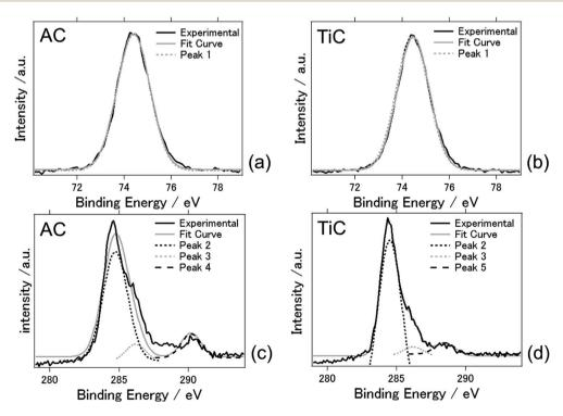
Fig. 5 X-ray photoelectron spectra of Al 2p of the air cathode after the electrochemical reaction for the air cathode composed of AC (a) and TiC (b). X-ray photoelectron spectra of C 1s of the air cathode after the electrochemical reaction for the air cathode composed of AC (c) and TiC (d).
