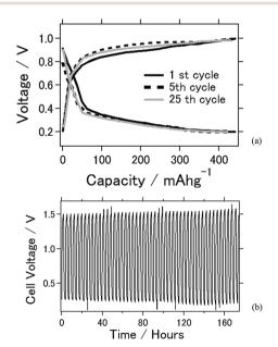
Fig. 2 (a) Charge–discharge curves of the aluminum–air battery with the TiC air cathode material at an applied current of  $\pm 0.5$  mA cm<sup>-2</sup>. (b) Voltage *versus* time plot of the aluminum–air battery with the TiC air cathode material at an applied current of  $\pm 2.0$  mA cm<sup>-2</sup>.
