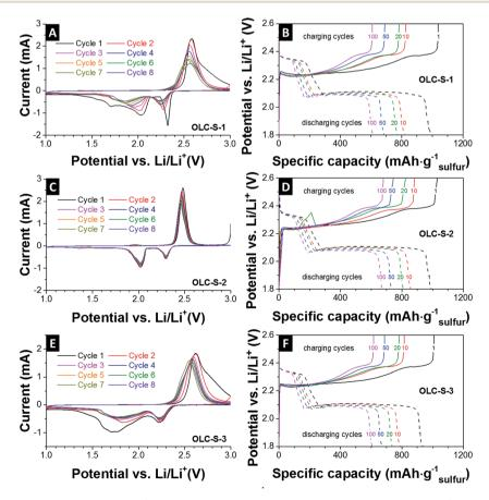
Fig. 4 Cyclic voltammograms at a rate of  $0.1 \text{ mV s}^{-1}$  and galvanostatic charge-discharge curves at 336 mA  $g^{-1}$  (0.2C) for charging and 168 mA  $^{-1}$  (0.1C) for discharging within the potential window of 1.8 V to 2.6 V versus Li/Li $^+$  of (A and B) OLC-S-1, (C and D) OLC-S-2, and (E and F) OLC-S-3.
