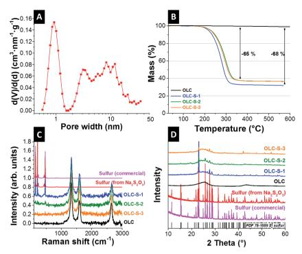
Fig. 3 (A) Pore size distribution of OLC calculated from QSDFT assuming slit pores, (B) sulfur contents from TGA, (C) Raman spectra (633 nm excitation wavelength) and (D) X-ray diffractograms of carbon onions and carbon onion/sulfur hybrids.
