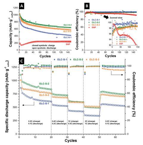
Fig. 5 Cycling performance (0.2C charge, 0.1C discharge) for the (A) specific capacity and (B) Coulombic efficiency (inset shows the zoomed range of 92–100%). (C) Rate capability study of the carbon onion/sulfur hybrid and sulfur nanoparticle (SNP) cathodes.
