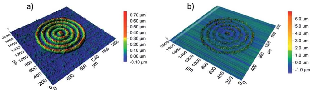
**Fig. 17** A comparison of the topography of (a) thermally and (b) photonicallly sintered silver molecular ink traces analyzed from optical profilometry. [Reprinted with permission from ref. 231 Copyright © American Chemical Society.]
