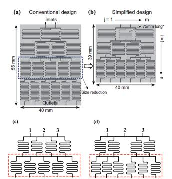
Fig. 2 Comparisons of a tree-shape network and the simplified design. (a) A tree-shape network and its overall geometrical sizes. (b) A simplified design of the tree-shape network in (a) and the reduced overall sizes (reproduced from ref. 82 with permission from Elsevier). (c) and (d) Partial enlargements of the splitting network in (a) and (b), respectively. Note that the simplified network in (b) obtains six concentrations in three stages as compared to four stages in (a).
