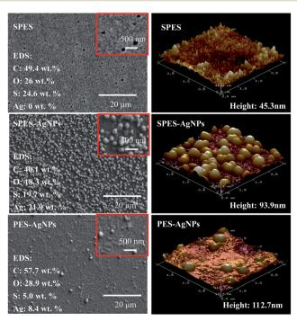
Fig. 2 SEM and AFM results of the SPES membrane; SPES-AgNPs membrane; and PES-AgNPs membrane.
