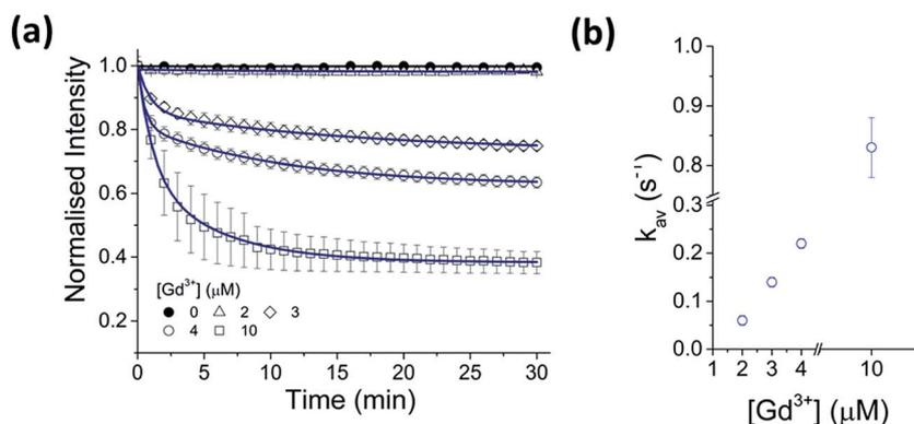
Fig. 2 Kinetics of CdTe 580 quenching induced by Gd<sup>3+</sup>. (a) Normalized variation in the fluorescence intensity of CdTe 580 QDs as a function of time in the absence and presence of 2 μM, 3 μM, 4 μM and 10 μM Gd<sup>3+</sup>. The solid lines represent fits to linear (black) and exponential decay (blue) functions. (b) The corresponding variation in the average quenching decay rate as a function of Gd<sup>3+</sup> concentration. Data are expressed as the mean ± SEM.
