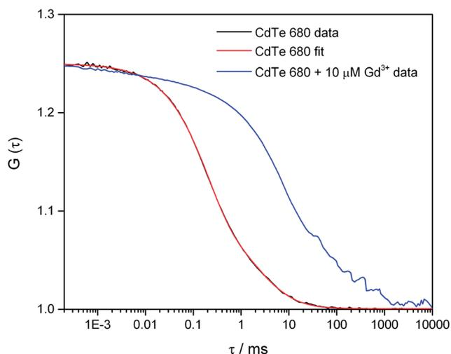
Fig. 5 Fluorescence correlation spectroscopy of CdTe 680 QDs in the absence and presence of  $\text{Gd}^{3+}$ . The correlation curve,  $G(\tau)$  of 25 nM CdTe 680 QDs in the absence of  $\text{Gd}^{3+}$  (black line) can be fitted (red line) using eqn (2). The fitting parameters are  $N = 4.01$ ,  $\tau_D = 1.985$  ms,  $F = 0.626$ ,  $\tau_{\text{dark}} = 0.197$  ms, and  $\beta = 0.793$ . Addition of  $10 \mu\text{M}$   $\text{Gd}^{3+}$  results in a pronounced shift to longer lag times.
