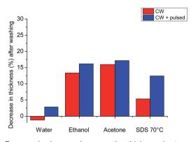
Fig. 2 Decrease in plasma polymer coating thickness due to exposure to different solvents and conditions. Positive values represent a percentage thickness decrease relative to the dry coating thickness. Error bars are present but appear small at this scale.
