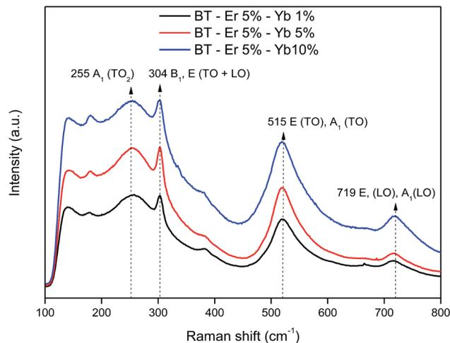
Fig. 3 Raman spectra for bare BaTiO<sub>3</sub> and BaTiO<sub>3</sub> doped with different concentrations of Er<sup>3+</sup> and Yb<sup>3+</sup> ions.
