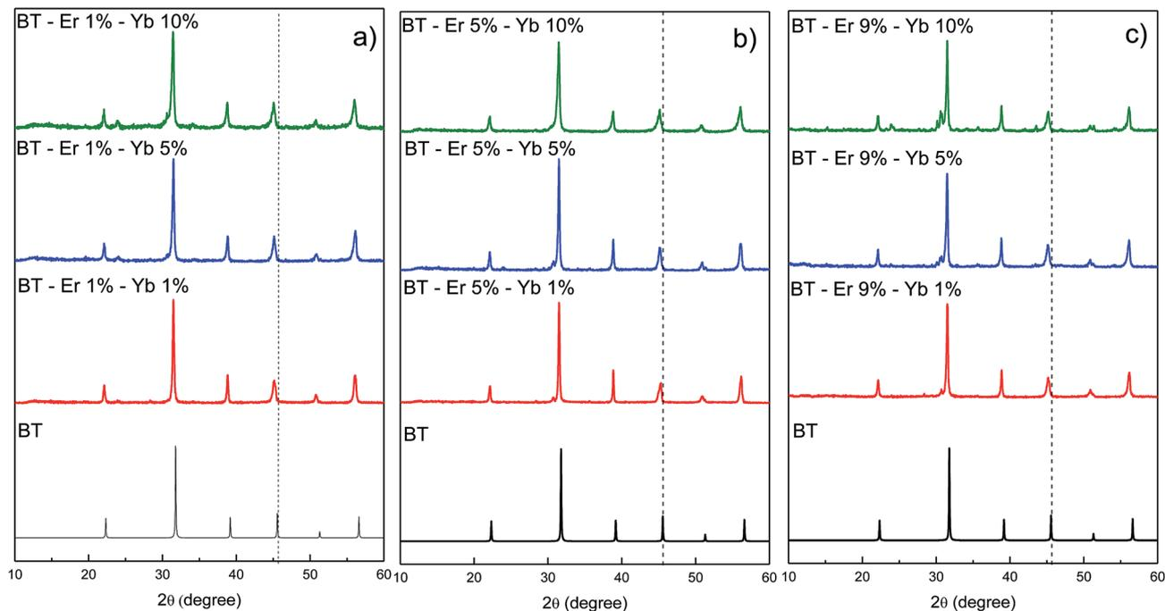
Fig. 1 XRD patterns of the BaTiO<sub>3</sub> doped with different contents of Er<sup>3+</sup> and Yb<sup>3+</sup> ions.
