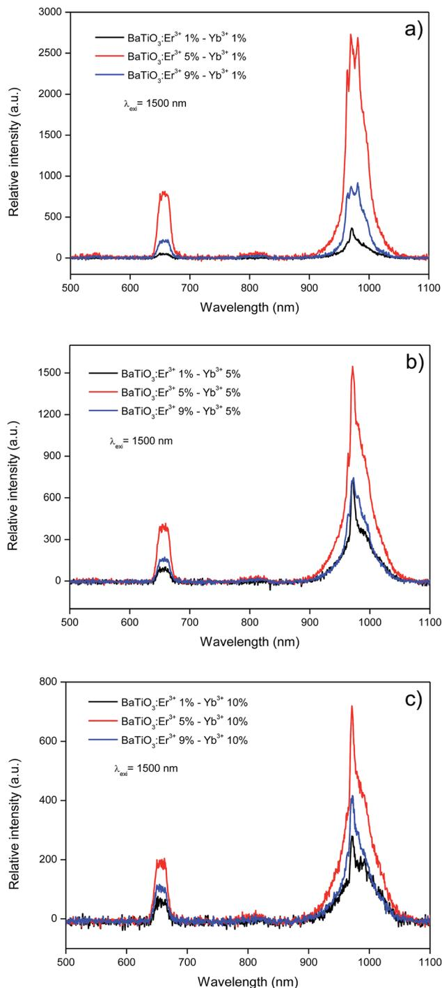
Fig. 6 Up-conversion spectra (excitation at 1500 nm) for BaTiO<sub>3</sub>:Er<sup>3+</sup> and Yb<sup>3+</sup> contents.
