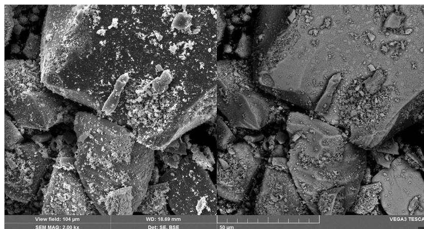
Fig. 4 SEM micrography for a BaTiO<sub>3</sub>:Er<sup>3+</sup> 5%–Yb<sup>3+</sup> 1% sample. Right: Backscattering and Left: secondary electrons.
