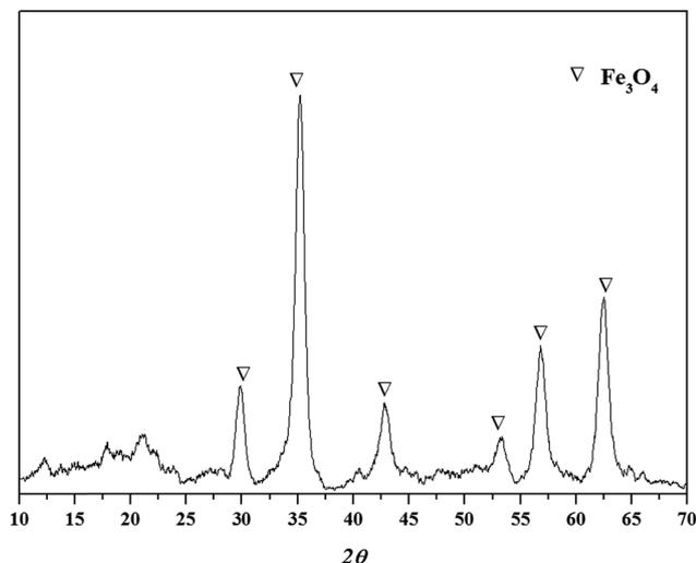
Fig. 2 XRD spectrum of the TW/Fe<sub>3</sub>O<sub>4</sub> composite.
