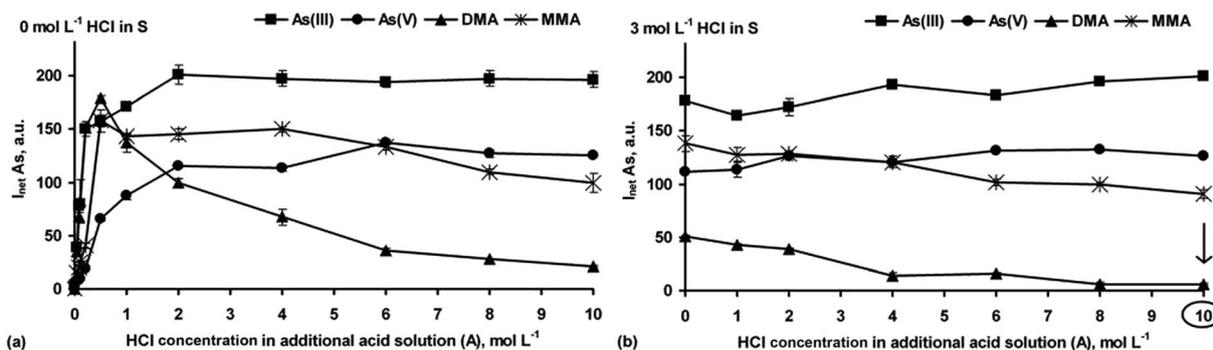
Fig. 1 Effect of acidity related to the HCl concentration in the additional acid (A) solution on the responses of As(III), As(V), DMA and MMA during arsine generation using a 1.0%  $\text{NaBH}_4$  (R) solution. The simple S solutions of the As species ( $20 \text{ ng g}^{-1}$  each) were used (acidification with HCl was omitted) (a) or they were acidified with HCl to  $3 \text{ mol L}^{-1}$  (b).
