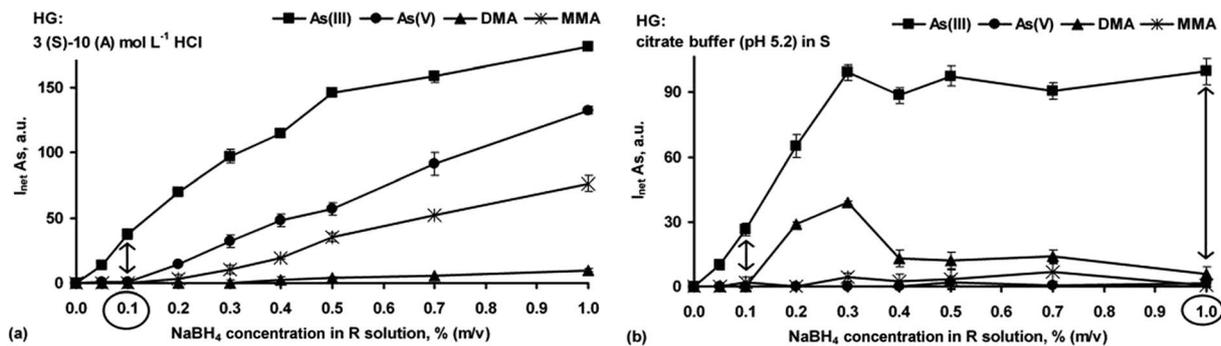
Fig. 3 Effect of the  $\text{NaBH}_4$  concentration on the measurements of As(III), As(V), DMA and MMA ( $20 \text{ ng g}^{-1}$  each) by HG-ICP OES using HCl (a) or a citrate buffer (pH 5.2) (b) for the HG reaction media.  $I_{\text{net}}$ : the average net intensity of the As line for  $n = 3$  measurements (S, A, R: sample, additional acid, reductant solutions).
