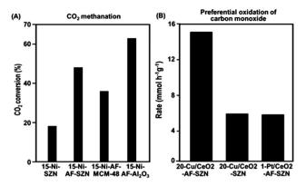
Fig. 4 (A) Conversion of CO<sub>2</sub> to methane over Ni supported on various kinds of supporting materials (reaction conditions: GHSV =  $17000 \text{ mL h}^{-1}\text{ g}^{-1}$ , H<sub>2</sub>: CO<sub>2</sub> molar ratio = 4:1, 300 °C, 1 atm). (B) Rate of CO conversion over Cu/CeO2 supported catalyst and Pt/CeO2 supported catalyst (reaction conditions: 130 °C, 50 mg of catalyst, 73 mL min<sup>-1</sup> of gas flow rate with a molar composition of  $CO/O_2/H_2/He = 0.7/0.8/63.0/34.9$ , 1 atm).
