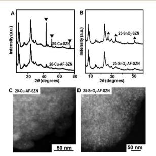
Fig. 2 (A and B) XRD patterns (bottom) and (C and D) STEM images of 20 wt% Cu and 25 wt%  $SnO_2$  supported AF-SZN samples. (A and B) XRD patterns (top) of 20 wt% Cu and 25 wt%  $SnO_2$  supported SZN samples are also displayed for comparison. The XRD peaks of metallic Cu and  $SnO_2$  are marked with an inverted triangle and a triangle.
