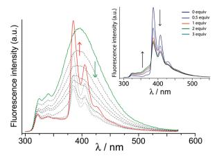
Fig. 3 Main figure: changes in fluorescence during addition of 3 to a solution of cage H (1 μM) in water resulting in formation of H·3: the cage fluorescence (green) is progressively quenched, and sensitised fluorescence from **3** (red) grows in. Inset: Restoration of fluorescence of cage **H**. and loss of sensitised pyrene fluorescence, on addition of cycloundecanone (3 equiv.) which displaces guest 3 from the cavity of H.
