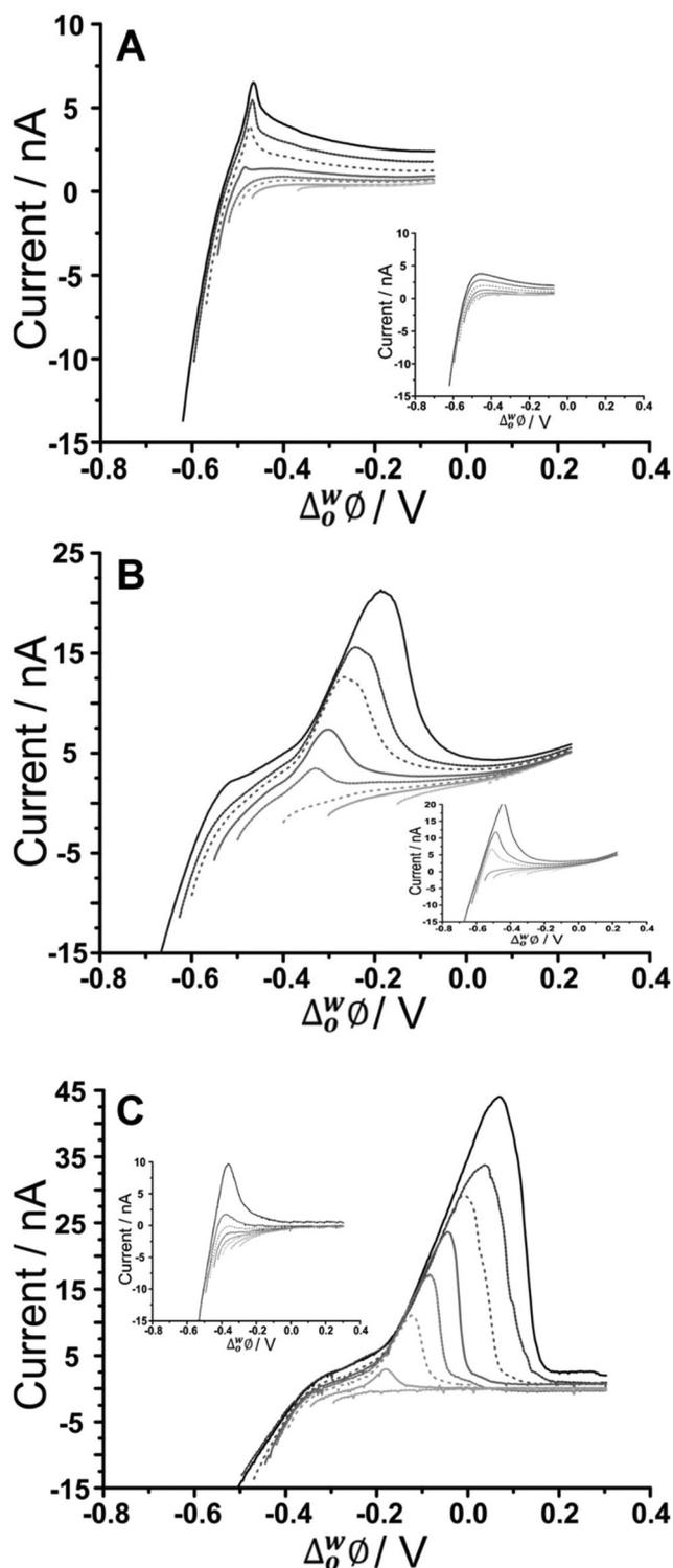
Fig. 3 AdSV in the presence and absence (inset) of  $500 \mu\text{g mL}^{-1}$  *U. pinnatifida* fucoidan, in aqueous phase of 10 mM NaOH (pH 12) following adsorption at different potentials. Adsorption time: 60 s, (A) Cell 1, (B) Cell 2, and (C) Cell 3 (Scheme 1). Scan rate:  $5 \text{ mV s}^{-1}$ .
