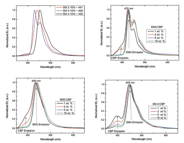
Electroluminescence spectra of SM 2-SM 4 (top left), and EL emission at various concentrations as noted
