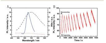
Fig. 6 (A) Absorption spectra of the PB film before (black curve) and after (red curve) the connecting of PB and Mg. The emission spectra of Ru@SiO<sub>2</sub> (blue curve); the sample was excited at 465 nm. (B) Fluorescence at 649 nm of the PB/Ru@SiO<sub>2</sub>/Nafion film as a function of time upon repeated discharging and charging cycles.
