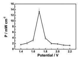
Fig. 3 Dependence of the power density on the cell voltage for the assembled Mg/PB battery in 0.025 M NaClO, 1 M KCl and 0.1 M phosphate buffer (pH 6) electrolyte, guiescent solution, under air.
