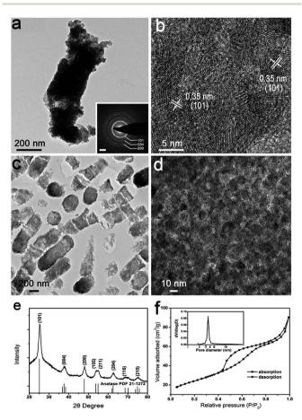
Fig. 2 Characterization of nanostructured anatase  $5\text{-TiO}_2$  annealed under air. (a) TEM image and corresponding SAED (inset) of representative rod-shaped structure. Scale bar in the inset is  $2~\text{nm}^{-1}$ . (b) HRTEM image of the rod-shaped structure. (c) Low and (d) high magnification microtome TEM images of anatase. (e) XRD pattern of nanostructured anatase. (f) Nitrogen adsorption and desorption isotherms and pore size distribution (inset).
