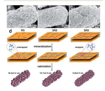
Fig. 3 Characterization of size-tunable anatase n-TiO $_2$  (n=1, 3, 5). SEM images of (a) 1-TiO $_2$ , (b) 3-TiO $_2$ , (c) 5-TiO $_2$ . (d) Schematic of confined space mineralization controlled by the number of repeating segments of R5.
