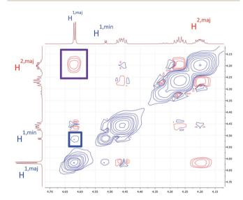
Fig. 6 A portion of the ROESY spectrum of 7a as observed in DMSO- $d_6$ . An NOE crosspeak is outlined in purple, while a conformational exchange (EXSY) crosspeak is outlined in blue.
