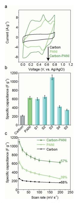
Fig. 4 Supercapacitor characterization. (a) Comparative CVs of carbon, PANI and carbon–PANI (composition S3) samples at a scan rate of 5 mV s $^{-1}$ . (b) Comparison of the specific capacitance performances of carbon, PANI and carbon–PANI nanocomposites (S1–S5) at various time intervals. (c) Variation of capacitance with scan rate for carbon, PANI and carbon–PANI nanocomposite (composition S3) samples.
