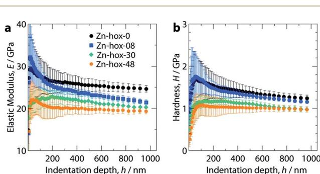
Fig. 4 Elastic moduli,  $E$  (a) and hardness,  $H$  (b) as a function of indentation depth,  $h$  along  $[110]$ . With increasing  $x$  in  $[\text{NH}_3\text{NH}_2]_{1-x}[\text{NH}_3\text{OH}]_x\text{Zn}(\text{HCOO})_3$ , the elastic modulus and hardness decrease monotonically due to reduced hydrogen bonding interactions upon substitution.
