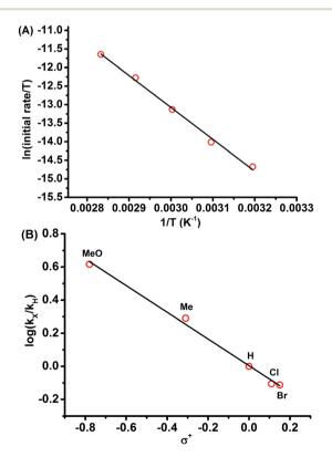
Fig. 1 (A) (top) Plot of ln(initial rate/T) vs. 1/T for the reaction between **1a** and NFSI in DCE, [**1a**] = 0.15 M, [NFSI] = 0.1 M, slope =  $-8.61 \times 10^3$ , y-intercept = 1.27  $\times$  10,  $r^2$  = 0.996. (B) (bottom) Hammett plot of  $\log(k_{\rm X}/k_{\rm H})$  vs.  $\sigma^+$  for the reaction of NFSI with para substituted diazo phenyl acetates 1 in DCE at 50 °C, [1] = 0.15 M, [NFSI] = 0.1 M, slope =-0.81, y-intercept =  $0.4 \times 10^{-2}$ ,  $r^2 = 0.995$
