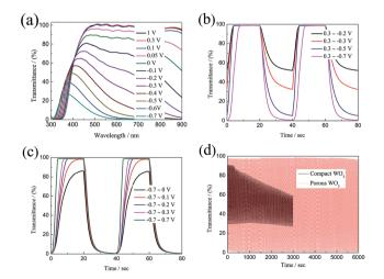
Fig. 4 (a) Transmittance of porous  $WO_3$  film as a function of applied potential. (b and c) *In situ* optical responses of porous  $WO_3$  films measured at 633 nm as a function of applied potential. (d) Cycle performance of the  $WO_3$  films measured in 0.5 M  $H_2SO_4$  for 6000 s.
