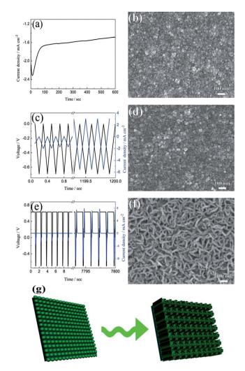
Fig. 1 The current–time responses and the corresponding SEM images for electrodeposited WO $_3$  films on ITO glasses: (a and b) continuous deposition, (c and d) pulsed electrodeposition without interval time, (e and f) pulsed electrodeposition with 1.1 s interval time between each pulse. (g) The formation process of porous and interconnecting flaky WO $_3$  film.
