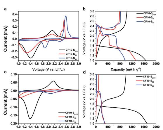
Fig. 3 The first CV scans at  $0.1 \, \text{mV} \, \text{s}^{-1}$  and the first GCD curves at 160 mA  $g^{-1}$  of CF10- $S_{pore}$ , CF10- $S_{60}$ , and CF10- $S_{90}$  in TEGDME electrolyte (a) and (b) respectively, and in EC/DEC electrolyte (c) and (d), respectively.
