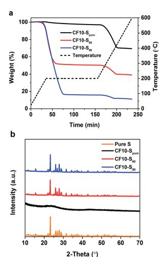
Fig. 2 (a) TGA curves and (b) XRD patterns of CF10-S<sub>pore</sub>, CF10-S<sub>60</sub> and CF10-S<sub>90</sub>.
