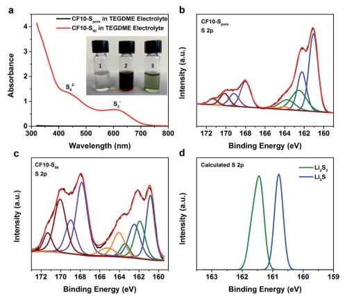
Fig. 4 (a) UV-Vis spectra of the TEGDME electrolyte used in CF10-S<sub>pore</sub> lithiation and the diluted TEGDME electrolyte used in CF10-S<sub>90</sub> lithiation, inset is photograph of the TEGDME electrolytes used in CF10-S<sub>pore</sub> and CF10-S<sub>90</sub> lithiation; XPS spectra of S 2p in (b) lithiated CF10-S<sub>pore</sub> and (c) lithiated CF10-S<sub>90</sub>; (d) predicted binding energies of sulfur in Li<sub>2</sub>S<sub>2</sub> and Li<sub>2</sub>S from DFT calculation.
