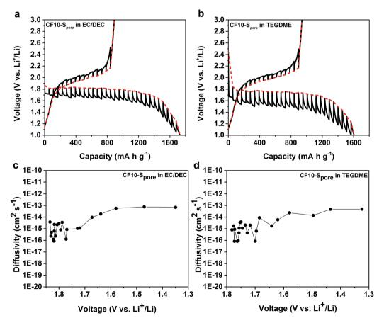
Fig. 6 GITT curves of CF10-S<sub>pore</sub> in (a) EC/DEC electrolyte and (b) TEGDME electrolyte; diffusivity of Li vs. potential calculated from the GITT data in (c) EC/DEC electrolyte and (d) TEGDME electrolyte.
