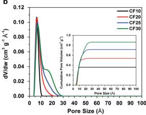
Fig. 1 (a) Type-I nitrogen adsorption—desorption isotherms and (b) pore size distributions (cumulative pore volume as inset) of the four different carbon fibres.
