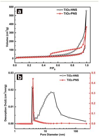
Fig. 3 (a) Nitrogen adsorption/desorption isotherms and (b) Barret–Joyner–Halenda (BJH) pore-size distribution curves of the  $TiO_2$ -HNSs and  $TiO_2$ -PNSs.
