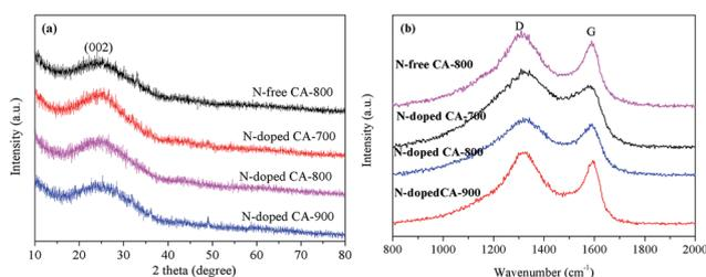
Fig. 3 XRD pattern (a) and Raman spectra (b) of N-free CA and N-doped CA.
