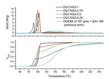
Fig. 1 Heat flow and calorimetric conversion during curing of DG174S3-X formulations at 10 °C min<sup>-1</sup> plotted with respect to the reference temperature of the DSC. The results from a previous analysis of the curing of DGEBA with 1MI are also shown.<sup>27</sup>
