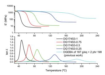
Fig. 6 DMA analysis of DG174S3-*r* formulations in comparison with a neat epoxy homopolymer formulation from a previous work.<sup>27</sup>
