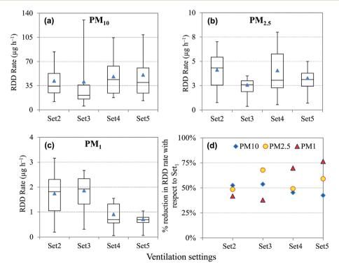
Fig. 6 Average RDD rate of (a) PM<sub>10</sub>, (b) PM<sub>2.5</sub> and (c) PM<sub>1</sub> during delay conditions at TIs in Set<sub>2</sub>, Set<sub>3</sub>, Set<sub>4</sub> and Set<sub>5</sub>. (d) Percentage reduction in incabin RDD rate during different ventilation settings with respect to on-road RDD rate during delay conditions at TIs. Please note that numbers on the x-axis represent the corresponding ventilation setting.
