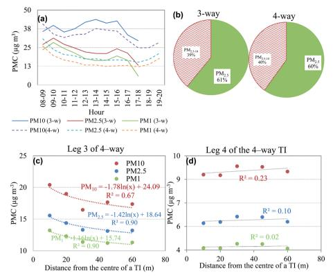
Fig. 4 (a) Diurnal profile of  $PM_{10}$ ,  $PM_{2.5}$  and  $PM_1$  at 3- and 4-way TIs. (b) Percentage contribution of fine and coarse particles to  $PM_{10}$ concentrations at 3- and 4-way TIs. Horizontal profile of  $PM_{10}$ ,  $PM_{2.5}$  and  $PM_{1}$  on (c) leg 3 and (d) leg 4 of a 4-way TIs.
