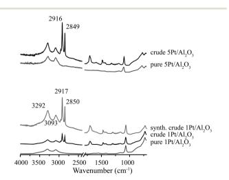
Fig. 7 ATR-IR spectra of spent 1Pt/Al<sub>2</sub>O<sub>3</sub> and 5Pt/Al<sub>2</sub>O<sub>3</sub> catalysts after APR of crude glycerol and glycerol solution.
