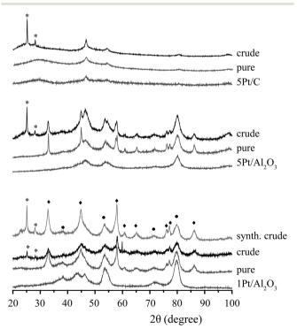
Fig. 6 XRD patterns of 1Pt/Al<sub>2</sub>O<sub>3</sub>, 5Pt/Al<sub>2</sub>O<sub>3</sub> and 5Pt/C catalysts before and after APR of crude glycerol, pure glycerol and synthetic crude glycerol mixture (glycerol/methanol/Na oleate); alumina (●), boehmite (\*) and newly formed adsorbed species (\*).
