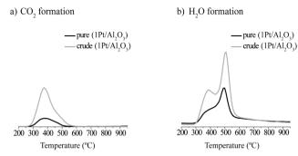
Fig. 5 a) CO<sub>2</sub> and b) H<sub>2</sub>O formation during thermogravimetric analyses of a spent 1Pt/Al<sub>2</sub>O<sub>3</sub> catalyst after the APR of pure (black) and crude (gray) glycerol.
