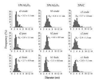
Fig. 3 Particle size distribution of the fresh and spent catalysts after pure glycerol APR and after crude glycerol APR for: (a) 1Pt/Al<sub>2</sub>O<sub>3</sub>, (b)  $5Pt/Al_2O_3$  and (c) 5Pt/C catalysts.  $D_m$  = mean particle size.
