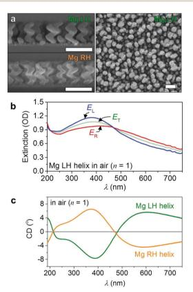
Fig. 2 Mg nanohelices. (a) SEM images of Mg LH (left-top panel) and RH (left-bottom panel) nanohelices. The right panel shows the top view of the array of the Mg LH nanohelices (scale bar: 200 nm). (b) Extinction spectra of the Mg LH nanohelices in air in response to the unpolarised light ( $E_T$ , green) and the circularly polarised light (LCP:  $E_{\rm L}$ , blue and RCP:  $E_{\rm R}$ , red). (c) CD spectra of the 178 nm thick film containing LH (green) and RH (orange) Mg nanohelices in air.
