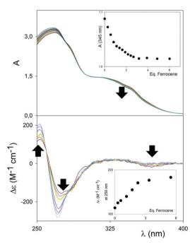
Fig. 2 Top: UV titration of metal-linked macrocycle (RR)-7 ( $2.5 \times 10^{-5}$  M) with ferrocene in MeCN at 25 °C. Inset: Titration profile vs. ferrocene added equivalents at 345 nm. Bottom: CD titration of macrocycle (RR)-7  $(1 \times 10^{-5} \text{ M})$  with ferrocene in MeCN at 25 °C. Inset: Titration profile vs. ferrocene added equivalents at 250 nm.
