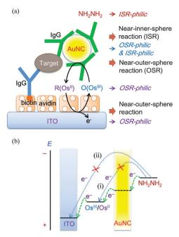
Fig. 1 (a) Schematic of an immunosensor using outer-sphere to innersphere electrochemical-nanocatalytic (EN<sub>c</sub>) redox cycling. (b) Schematic of three-step electron transfer related to EN<sub>c</sub> redox cycling (green lines) and unwanted electron transfer (sky-blue lines). The applied potential, the formal potentials of  $Os^{III}(bpy)_2Cl_2^+/Os^{II}(bpy)_2Cl_2$  and hydrazine, and the potential of the Au nanocatalyst (AuNC) (horizontal lines) are positioned in order of potential.
