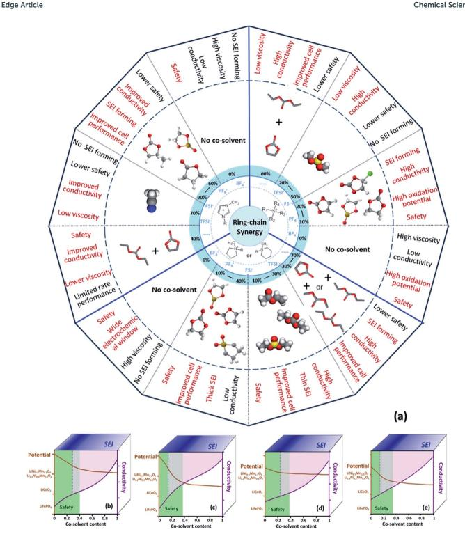
Fig. 8 (a) Illustration of representative electrolyte systems based on ionic liquids for lithium batteries with the corresponding characteristics. Semi-quantitative threshold of the properties of the electrolyte systems: (b) ring-like ionic liquid and ring-like cosolvent, (c) ring-like ionic liquid and chain-like cosolvent, (d) chain-like ionic liquid and ring-like cosolvent and (e) chain-like ionic liquid and chain-like cosolvent. 11,13-17,19,24,34,46-78
