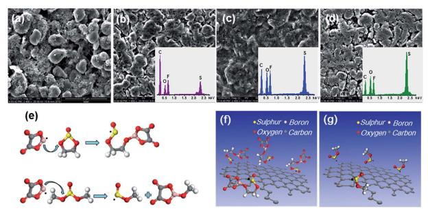
Fig. 5 (a) SEM image of the MCMB anode before cycling. SEM and EDS of the SEI layer on the MCMB anode in (b) LiODFB-Pyr<sub>1,2O1</sub>TFSI, (c) LiODFB-Pyr<sub>1,2O1</sub>TFSI/ES, and (d) LiODFB-Pyr<sub>1,2O1</sub>TFSI/DMS electrolytes after 10 cycles. Schematic illustration of the synthesis route to SEI: (f) ES; (g) DMS, with the prime reactions (e).
