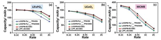
Fig. 7 Rate capability of the Li/LiFePO<sub>4</sub> (a), Li/LiCoO<sub>2</sub> (b) and Li/MCMB (c) cells with LiODFB-Pyr<sub>1,2O1</sub>TFSI/ES, LiODFB-Pyr<sub>1,2O1</sub>TFSI/DMS, LiODFB-EC/DEC or LiPF<sub>6</sub>-EC/DEC electrolytes.
