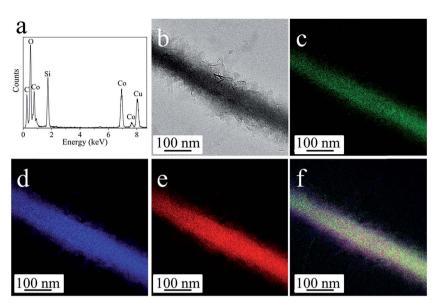
Fig. 2 (a) EDX spectrum taken from a single nanobelt, in which the C and Cu signals originate from the TEM grid. (b-f) EFTEM images: (b) zero-loss image, (c) Co L-edge, (d) Si L-edge, (e) O K-edge, (f) overlapping of Co, Si and O maps.
