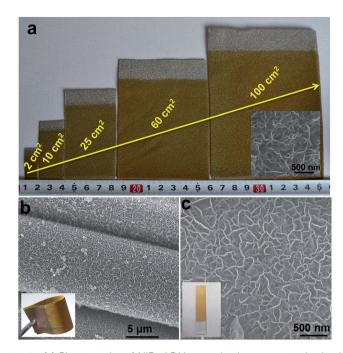
Fig. 5 (a) Photographs of NiFe-LDH nanoplatelet arrays synthesized on foam nickel substrates at various scales (inset: the SEM image of the NiFe-LDH sample on the 100 cm<sup>2</sup> substrate); synthesis time for all the samples is 300 s at room temperature. SEM images for the NiFe-LDH nanoplatelet arrays on (b) a conducting cloth and (c) FTO substrate (inset: their corresponding photographs).
