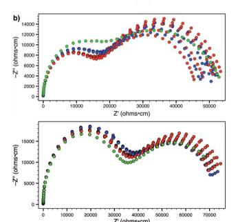
Fig. 7 (a) Current response from 300 mV applied potential to 14 (red) and 19 (blue) in a symmetric lithium metal cell. (b) AC impedance spectra collected during 24 hour operation of Li(s)|electrolyte|Li(s) symmetric cells. Top: Polymer 14. Bottom: Polymer 19. Red data represents impedance spectra taken without constant applied voltage. Blue data represents spectra taken with 300 mV applied voltage. Green data represents the final spectrum taken after the experiment.
