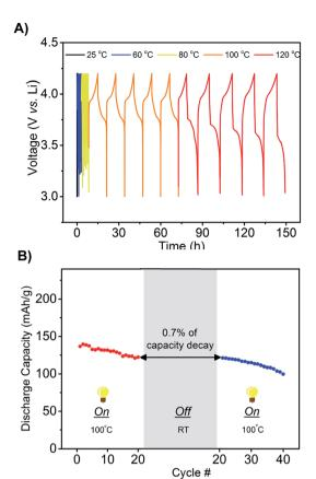
Fig. 4 (A) Charge–discharge voltage profile of the thermally responsive ionic liquid electrolyte in a (Li, LiCoO $_2$ , mono-(C $_6$ ) $_3$ PC $_{10}$ -TFSI, 1.6 M LiTFSI) cell (current rate C/7). Measurements are presented by heating from 25 to 120 °C and five cycles were measured at each temperature. (B) Demonstration of battery working only at high temperature and retain capacity at room temperature.
