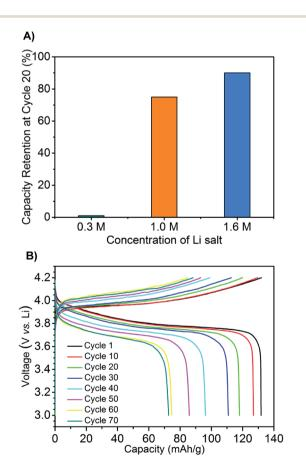
Fig. 3 (A) The percent of specific capacity of cycle 1 at cycle 20 for 0.3 M, 1.0 M and 1.6 M compositions respectively. (B) Galvanostatic charge-discharge cycling for 1.6 M LiTFSI composition, current rate at C/7.
