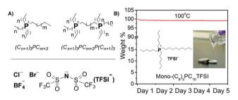
Fig. 1 Chemical structures of ionic liquids under investigation. (A) lonic liquids investigated in pre-screening; (B) picture and long-term thermal stability of the selected ionic liquid (mono- $(C_6)_3$ PC $_{10}$ TFSI) for battery testing.
