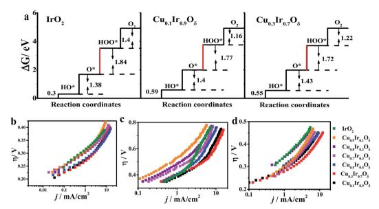
Fig. 7 (a) Standard free energy diagram for the OER in  $IrO_2$ ,  $Cu_{0.1}Ir_{0.9}O_\delta$  and  $Cu_{0.3}Ir_{0.7}O_\delta$ . (b-d) Tafel plots in acidic, neutral and basic solutions, respectively. The curves are iR-corrected in the acidic ( $\sim$ 18  $\Omega$ ), neutral ( $\sim$ 15  $\Omega$ ) and basic ( $\sim$ 28  $\Omega$ ) solutions, respectively. The catalyst mass loading was  $\sim$ 0.2 mg cm<sup>-2</sup> for all electrodes.
