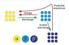
Fig. 3 Schematic diagram of phase transitions in Al-doped Li $_4$ Ti $_5$ O $_{12}$  under different discharging cutoffs, in which  $\alpha$  is the delithiated phase,  $\beta$  is the lithiated phase, and  $\beta'$  is the lithiated phase discharged to a very low cutoff potential.
