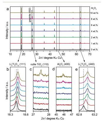
Fig. 5 (a) XRD patterns of Al-doped Li<sub>4</sub>Ti<sub>5</sub>O<sub>12</sub> with different doping levels. In the precursor, the amount of Al<sub>2</sub>O<sub>3</sub> is varied from 0 wt% to 10 wt%. Enlarged XRD patterns of (b)  $Li_4Ti_5O_{12}$  (111), (c) rutile  $TiO_2$  (110), (d)  $Al_2O_3$  (400), (e)  $Li_4Ti_5O_{12}$  (440) peaks. During the XRD measurements, ca. 5% graphite is mixed into the samples to calibrate the position of peaks.
