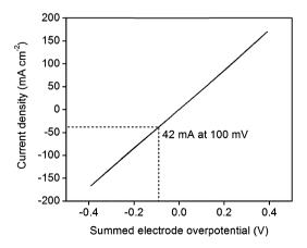
Fig. 8 IR-corrected polarization curve of a 46 wt% Pt-CNT-CsH $_2$ PO $_4$  composite electrode at 1 mV s $^{-1}$ , showing high current density at low overpotentials for both proton reduction and hydrogen oxidation.
