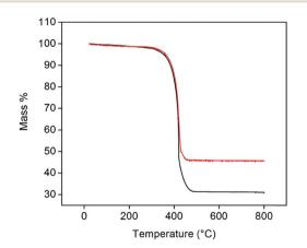
Fig. 3  $\,$  TGA profiles of 30 (black) and 46 wt% (red) Pt-CNTs (measured under flowing air at a heating rate of 2  $^{\circ}C$  min  $^{-1}$ ).
