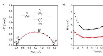
Fig. 7 Symmetric cell impedance measurements Pt-CNT based electrodes prepared by strategy 2: (a) Nyquist plot for 46 wt% Pt-CNT-CsH $_2$ PO $_4$  composite after 4 hours (inset: equivalent circuit used for fitting) and (b) temporal evolution of the electrode resistance values of 30 wt% (black) and 46 wt% (red) Pt-CNT-CsH $_2$ PO $_4$  composites, showing higher stability in the electrolyte with higher Pt loading.
