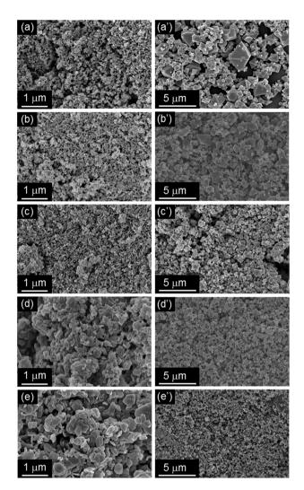
Fig. 2 SEM images of the solvent insoluble Cu-based precursors (Cubased precursors X, (a-e) and corresponding HKUST-1X (a'-e'). (a) X = 00.5, (b) X = 1, (c) X = 2, (d) X = 3, (e) X = 4.
