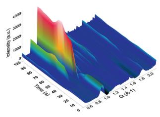
Fig. 6 Nucleation and growth of HKUST-1\_2 at room temperature as a function of time when the alcoholic solution containing BTC is added to the solution containing Cu-based precursors\_2. The ligand was injected at t=30 seconds. A SAXS-based diffraction pattern of HKUST-1\_2 as a function of time shows that nucleation starts within 5 seconds after addition of the organic linkers.
