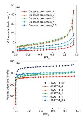
Fig. 5 N<sub>2</sub> adsorption isotherms of (a) the solvent insoluble Cu-based precursors (Cu-based precursors\_X) and (b) corresponding HKUST-1\_X with HKUST-1\_ref measured at 77 K.
