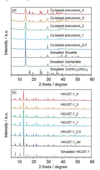
Fig. 3 XRD patterns of (a) the solvent insoluble Cu-based precursors (Cu-based precursors\_X) with simulated patterns for  $\text{Cu}_2(\text{OH})_3\text{NO}_3$  (rouaite and gerhardite) and  $\text{Cu}(\text{NH}_3)_4(\text{NO}_3)_2$  and (b) corresponding HKUST-1\_X with HKUST-1\_ref and simulated pattern for HKUST-1.
