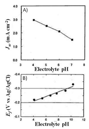
Fig. 18 (A) pH dependence of  $J_{sc}$  values ( $P_{in}=1$  sun) obtained for an aqueous DSSC sensitized with N719. Electrolyte: KI 0.50 M and I $_2$  25 mM; (B) dependence of the Fermi level electrochemical potential ( $E_f$ ) of the mesoporous TiO $_2$  electrode on the pH of the above reported electrolyte. The potential data were based on the measurement of the onset potential of dark cathodic current. Adapted and reprinted from ref. 138.
