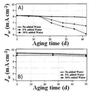
Fig. 17 Long-term stability ( $P_{\rm in}=0.015~{\rm mW~cm^{-2}}$ ) of DSSCs assembled with RTIL-based electrolytes ( $I_2$  10 mM in HMII) encompassing different H<sub>2</sub>O contents. Dyes: (A) N3; (B) [Ru(H<sub>2</sub>dcbpy)(mhdbpy)(NCS)<sub>2</sub>]. Adapted and reprinted from ref. 231.
