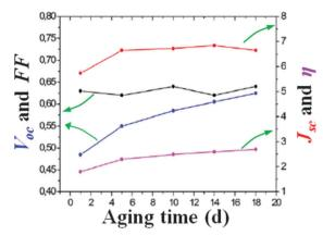
Fig. 20 Long-term stability under dark of DSSCs assembled with a fully agueous electrolyte (KI 4.0 M and I<sub>2</sub> 20 mM at pH 8.0) and a PEDOT counter electrolyte. Dye: V35. PV parameters were measured under  $P_{in} = 1$ sun. Adapted and reprinted from ref. 249
