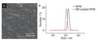
Fig. 3 (A) SEM image of NFMs cast onto a glass slide. (B) Hydrodynamic size distribution of NFMs measured by DLS.
