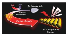
Scheme 1 Formation of AuNPCs via the controlled galvanic replacement of AgNPs with Au precursors.
