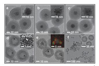
Fig. 1 TEM and HRTEM (insets) images of (a) (Fe<sub>3</sub>O<sub>4</sub>/Au)@(SiO<sub>2</sub>/Ni<sup>2+</sup>), (b)  $(Fe_3O_4/AuPt^{2+})@SiO_2$  and (c)  $(Fe_3O_4/Au)@(SiO_2/Pd^{2+})$  core@shell nanospheres and (d)  $Au@h-SiO_2$  (e)  $(Fe_3O_4/AuPt)@h-SiO_2$  (insets: EDX elementary maps, Au (red), Pt (green)) and (f) (Au/Pd)@h-SiO2 yolk@shell nanospheres, which were produced by treating the core@shell nanospehres with NaBH<sub>4</sub>.
