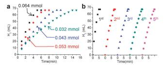
Fig. 4 Plots of volume of hydrogen generated vs. time for catalytic hydrolysis of AB (a) at various concentrations of the Ni@SiO2 catalyst and (b) during the recycling experiment.
