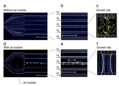
Fig. 5 Fluorescent flow tracer analysis: (a-c) normal cultivation conditions with equal flow rates inside all supply channels; (c) diffusive mass transport conditions inside the cultivation chambers; (d) air bubble is deployed at the fivefold channel junction resulting in (e) a temporary inhomogeneous laminar flow profile and different volume flows  $\Phi_1$ ,  $\Phi_2$ ,  $\Phi_3$ ,  $\Phi_4$  and  $\Phi_5$  and thus (f) laminar flow through the cultivation chambers (scale bar 25 µm).
