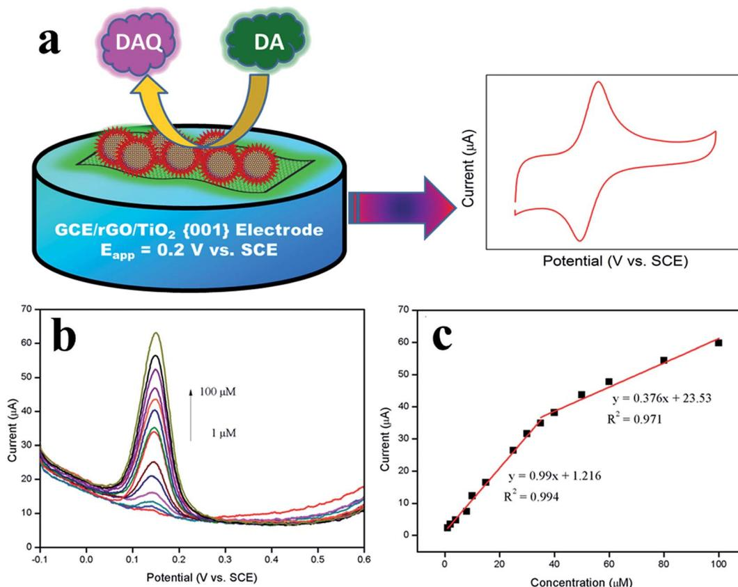
Fig. 13 (a) Mechanism for the electrocatalytic oxidation of dopamine at rGO/TiO<sub>2</sub> {001} modified GCE. (b) DPV obtained for rGO/TiO<sub>2</sub> {001} modified GCEs during the addition of 1, 2, 4, 8, 10, 15, 25, 30, 35, 40, 50, 60, 80, and 100 μM DA into the 0.1 M PBS (pH = 6.5). (c) Calibration plot observed for the oxidation peak current vs. concentration of DA. Reprinted with permission from ref. 123, Copyrights (2014) Nature publishing Group.
