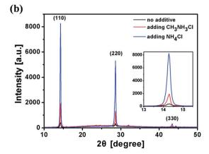
Fig. 2 UV-vis absorption spectra (a) and XRD patterns (b) for CH<sub>3</sub>NH<sub>3</sub>Pbl<sub>3</sub> films fabricated by using different additives.
