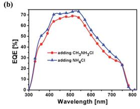
Fig. 4 J-V curves (a) and EQE spectra (b) for  $CH_3NH_3PbI_3$  solar cells fabricated by using different additives.
