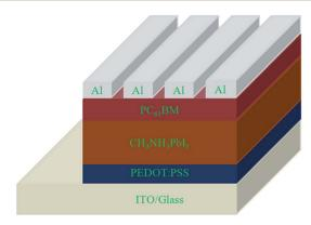
Fig. 1 Structure of CH<sub>3</sub>NH<sub>3</sub>PbI<sub>3</sub>/PC<sub>61</sub>BM solar cells.
